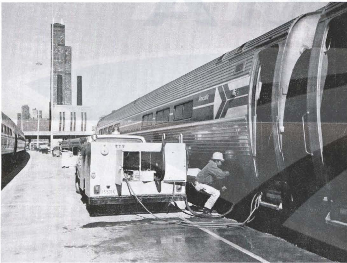
Mobile units use concrete ramps between tracks to reach cars for servicing. Roy Simmons works on an Amfleet car.
