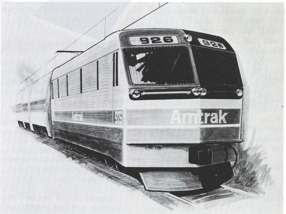
Amtrak's new four-axle electric locomotive will pull trains at up to 120 miles per hour.
