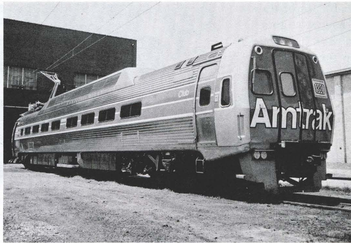
The refurbished Metroliners present a new and sleek profile to the public. The raised area on the roof houses components that had previously been located beneath the car.
