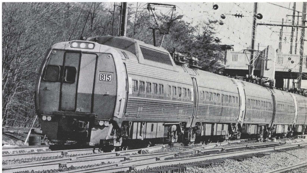
Metroliner, with one of the present modified cars on the head end, speeds toward Washington. The upgraded Metroliners will all have the elevated section in the center of the car roof.
